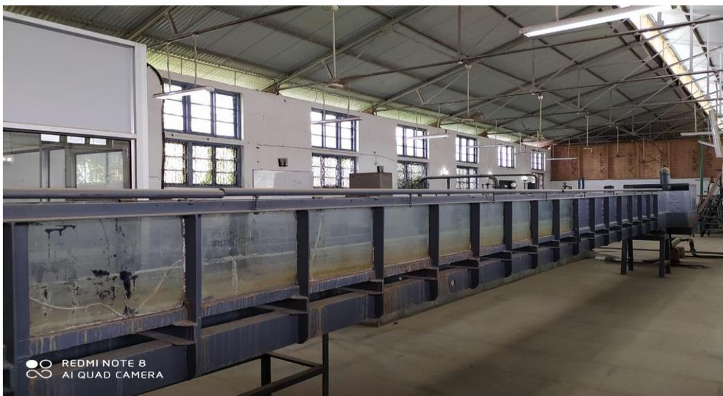
Rectangular Channel(flume) in the fluid mechanics Lab.
